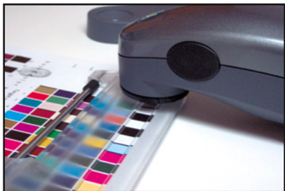
The ii has to be located in an unprinted area before you start measuring, otherwise the measuring will be faulty
