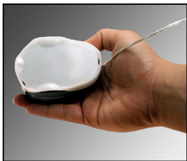
Positioning basICColor SQUID2 for ambient light measurement.
