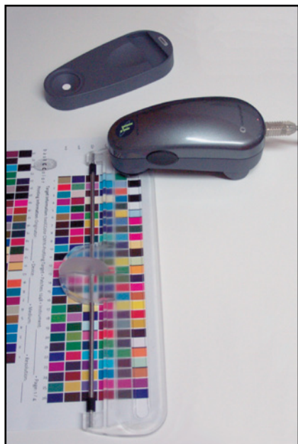
Positioning the gretagmacbeth Eye-One pro on the measurement ruler.
