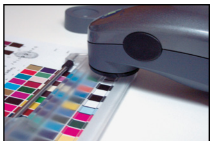
To identify the strip correctly the head of the Eye-One Pro has to be positioned in the white area if front of the first patch of the strip.
